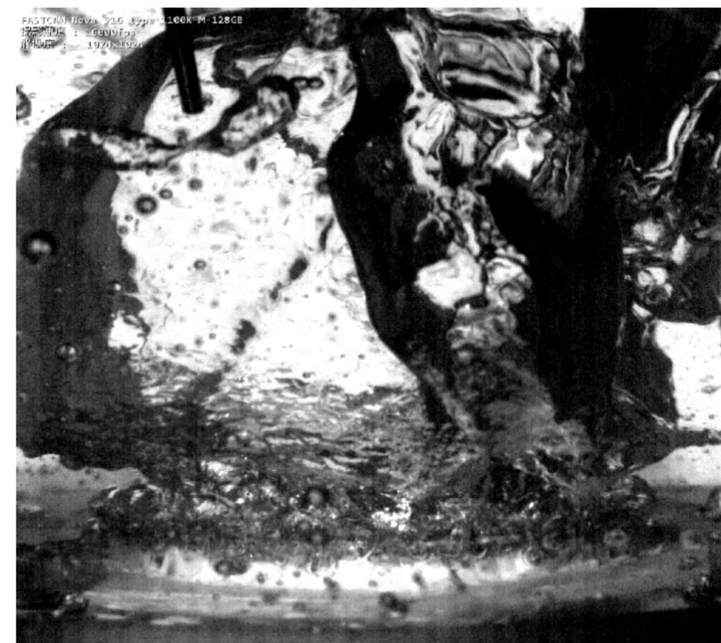
Figure 7: Near CHF boiling for small lattice: 1,992 kW/m²
