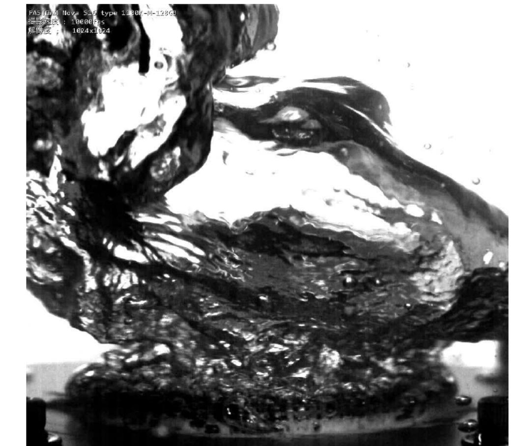
Figure 8: Near CHF boiling for large lattice: 2000 kW/m²
